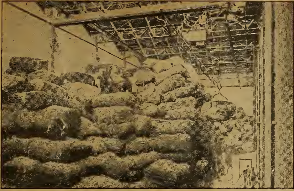
Old rags are the basis of roofing felt. There is a well-established rag market with definite grades and standards of quality
