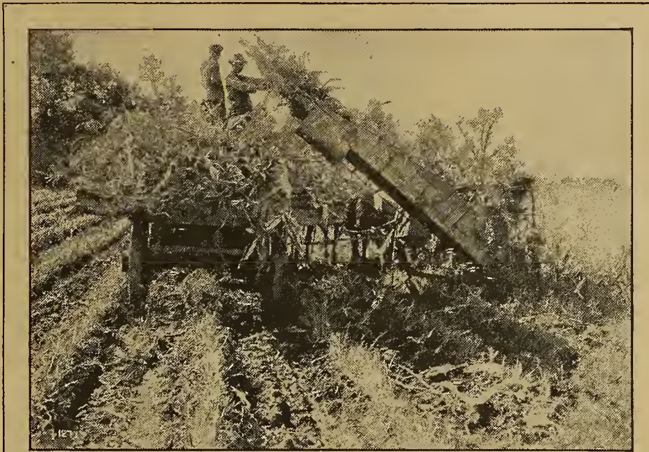
The elevator from the corn binder delivers the bundles to the wagon. The work goes quickly and nobody sweats blood
