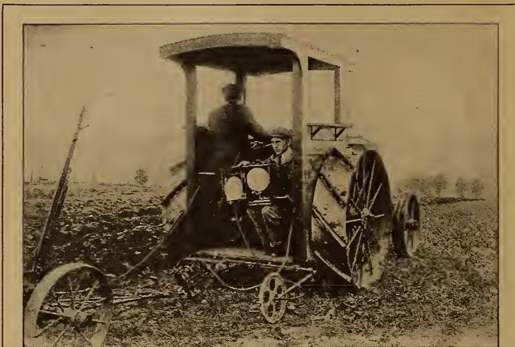
The instrument with the large white dials is a dynamometer and registers the power required to pull the plows
