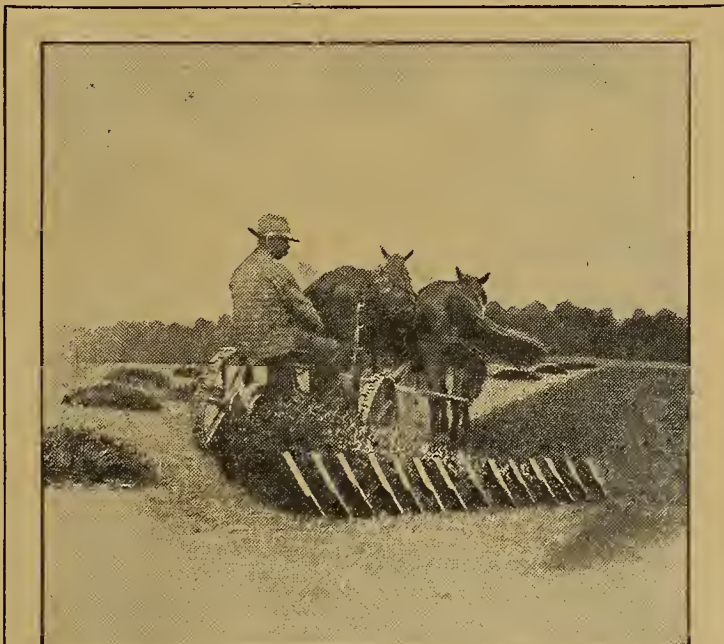
Here is one style of buncher used in connection with a mower to harvest clover for seed
