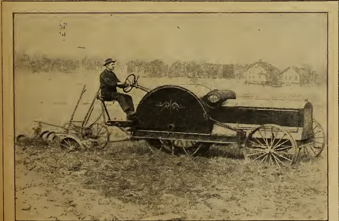
Here is one of several tractors that have adopted a close-fitting hood to keep dust and grit out of the engine. Also note the low-down construction
