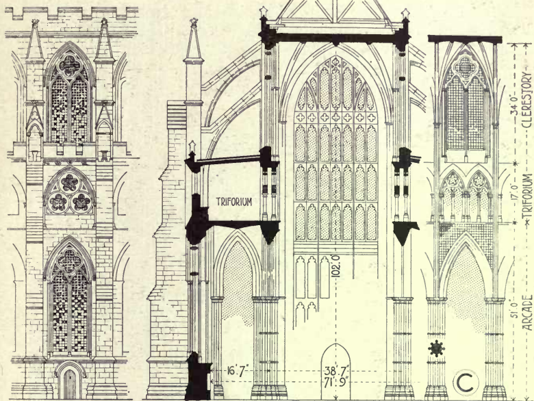
A EXTERNAL BAY NORTH SIDE SCALE FOR SECTIONS 0 5 10 20 30 40 50 FEET B SECTION INTERNAL BAY NORTH SIDE
