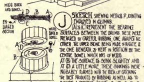
(J) SKETCH SHOWING METHOD JOINTING ENJOINED IN COLUMNS
