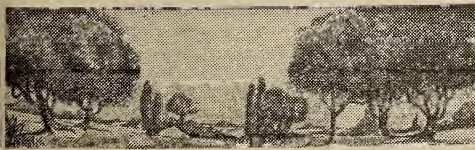
80-line screen half-tone on copper. Used with ordinary glazed or calendered paper.
