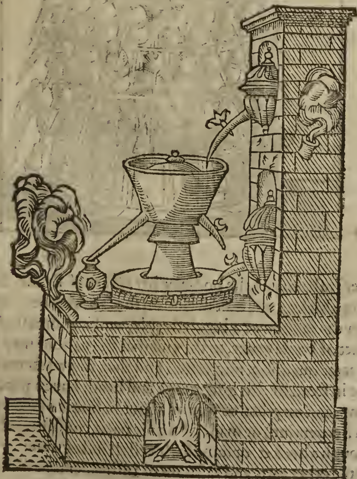
The Venetians distill their water in such an Instrument: The furnace is round, and containeth on euerie side, round about it, manie earthen vessels, glased within, and
