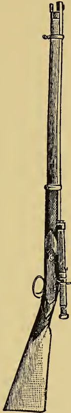
Fig. 68. Whitworth Military Rifle with Davidson Telescope.
