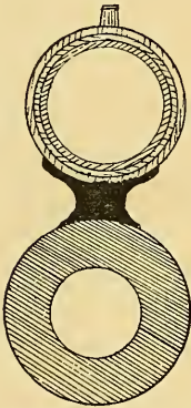
Fig. 70.—Muzzle View on long-range rifle showing rib, telescope tube and cells holding object lens and deflecting prism.
