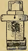
Fig. 33.—Sight on an ancient cross-bow in Tower of London, showing Peep Sight and Lateral Sliding-bar Wind Gauge.
