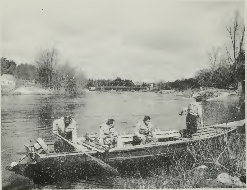
MEASURING THE RIVER FLOW Boat and crew equipped for stream flow measurements
