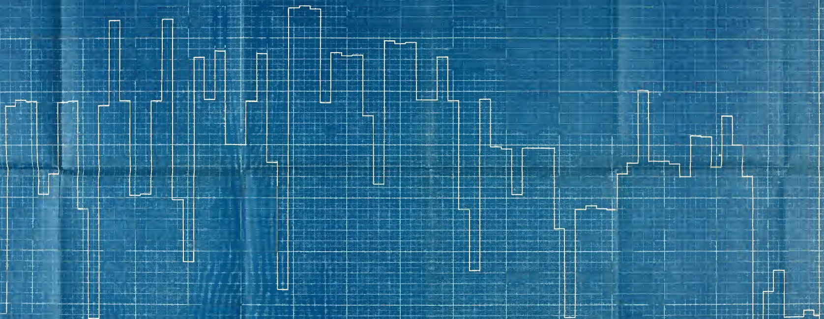
POWER PLANT AVERAGE LOAD CURVE. PROPOSED DANVILLE - TERRE HAUTE INTERURBAN RAILWAY. ARMOUR INSTITUTE OF TECHNOLOGY CHICAGO, ILL. A. H. Oswald - Engrs. - H. M. Shapiro May 8, 1916.
