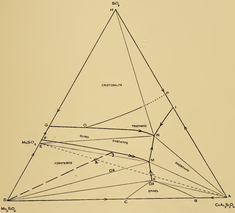
FIG. 4.—Equilibrium diagram of the system: anorthite, forsterite, silica, after Andersen, Am. Jour. Sci. (4), XXXIX (1915), 437.
