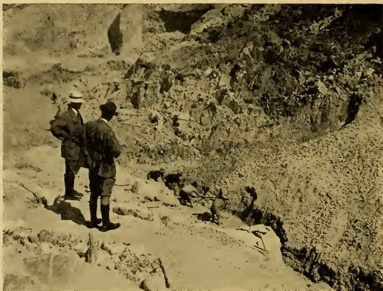
FIG. 24.—Diamond mining at Cadette's mine. The clay and materials of lesser specific gravity are washed away by running water while the diamonds and other heavy pebbles remain behind and become concentrated.
