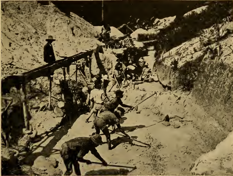
FIG. 25.—Stirring up the mortar-like mass of diamond-bearing clay and gravel
