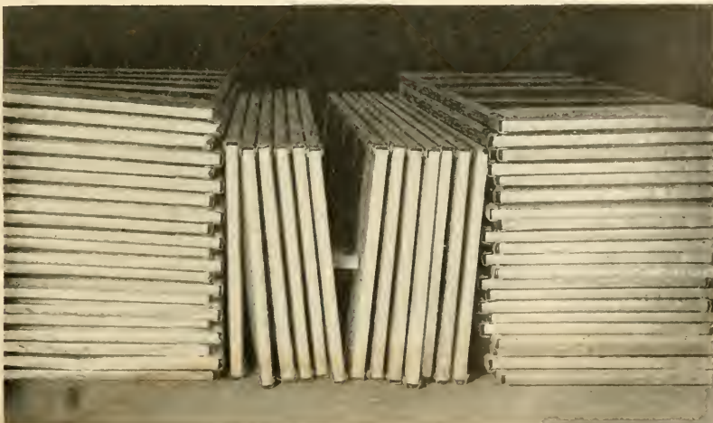
Shipment Packed in Metal Crates. Space Occupied about One-Half that of Wooden Crates. Patent Applied For.
