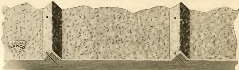
Above Cut shows where to Nail V-Crimp Roofing.
