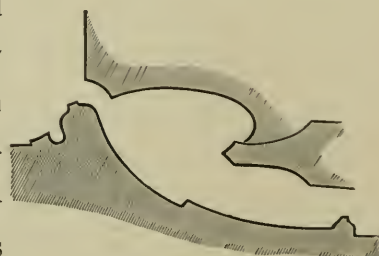
SECTION OF JAMB AND SILL.
