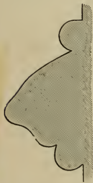
BAND TO NAVE-PIERS. PERPENDICULAR.
