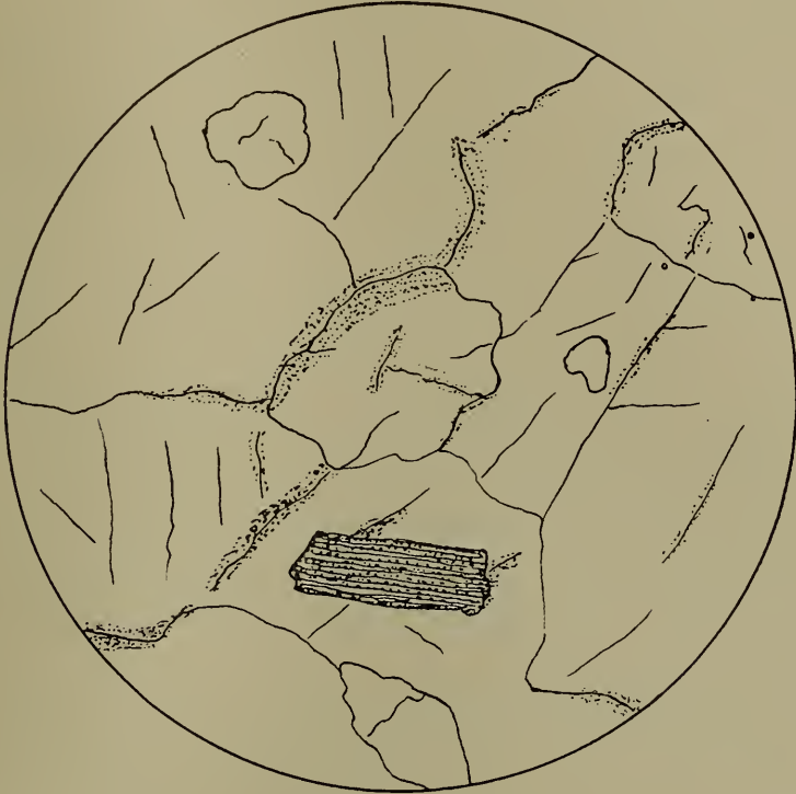
Fig. 11 The yellow Mohegan granite, showing concentration of limonite along the borders and in the cleavage cracks of the mineral particles
