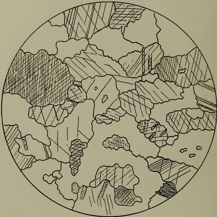
Fig. 15 Gouverneur marble in thin section, showing the irregular boundaries between the particles and firmly interlocked texture. Enlarged 25 diameters
