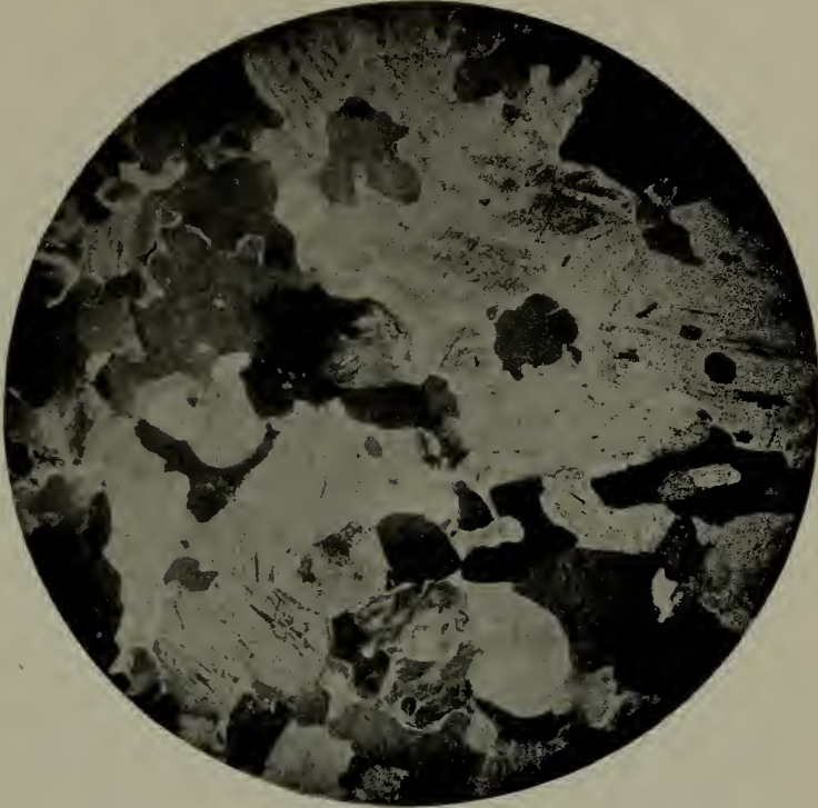
Photomicrograph of green syenite, Ausable Forks. Mostly feldspar, with some quartz and pyroxene. Enlarged 22 times.
