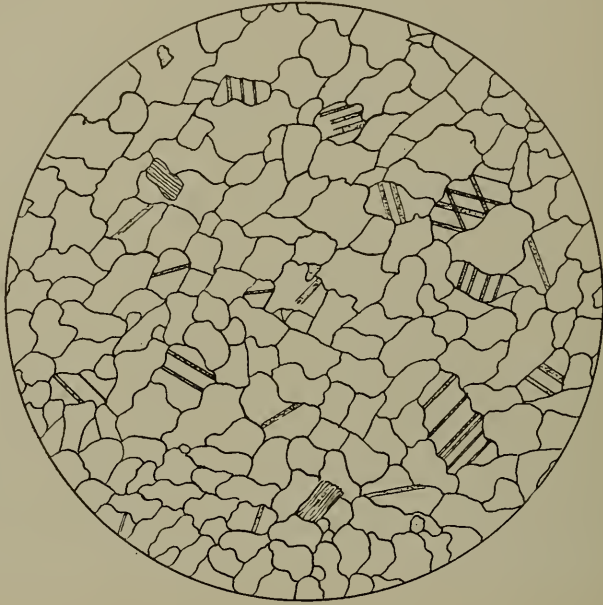
Fig. 17 South Dover marble in thin section. Enlarged 10 times
