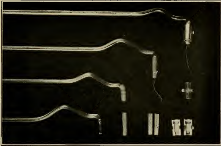
3. Assembly, consisting of glass manometer, rubber connecting tube, and metal clamp, by which a single tomato root can be attached to a recording apparatus and its secretion forces measured. (Photograph by J. A. Carlisle.)
