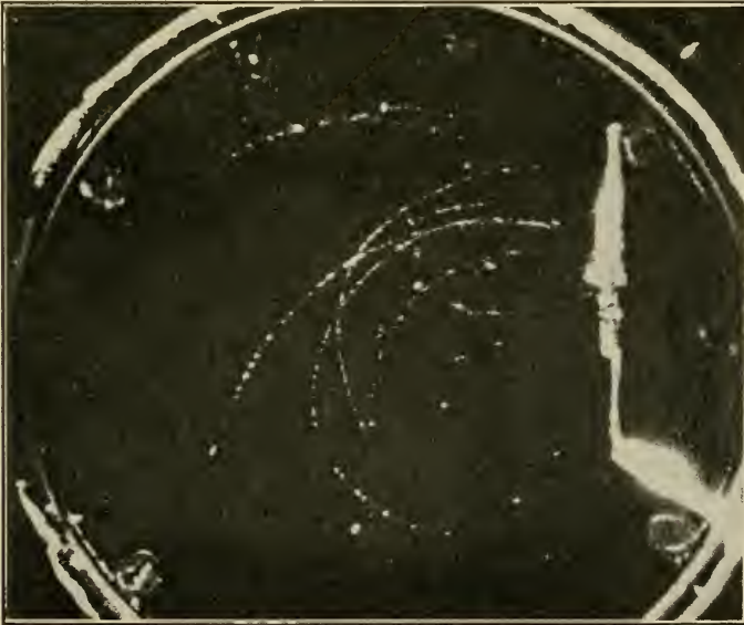
2. Cloud chamber photograph showing the emission of positrons by radioactive nitrogen which was produced when the carbon plate shown at the right was bombarded by 900,000 electron-volt protons. (Anderson and Neddermeyer.)
