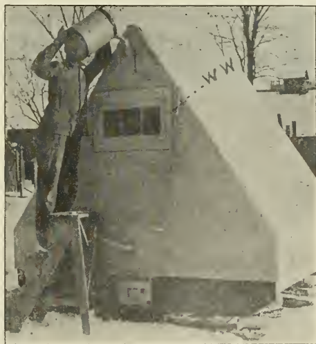
FIG. 74.— Filling. A small hole should be punched in the cap of the oil can to insure an even flow of gasoline and steady flame.
