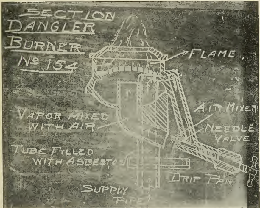
FIG. 68.—Cross section drawing of burner.
