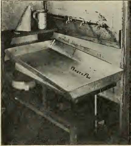
FIG. 107.—The interior arrangement for draining oil. Note edge of table at left for cleaning and trimming lamps.
