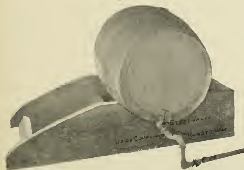
FIG. 106.—The oil barrel in position. The astral oil gives better results than the standard 150 test.
