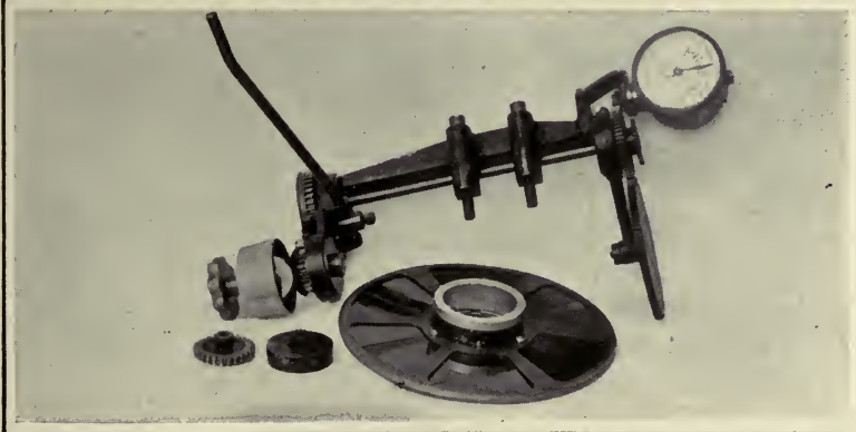
STANDARD MOTION-PICTURE PROJECTOR EQUIPPED WITH COLOR-WHEEL ATTACHMENT SHOWN IN LOWER VIEW
