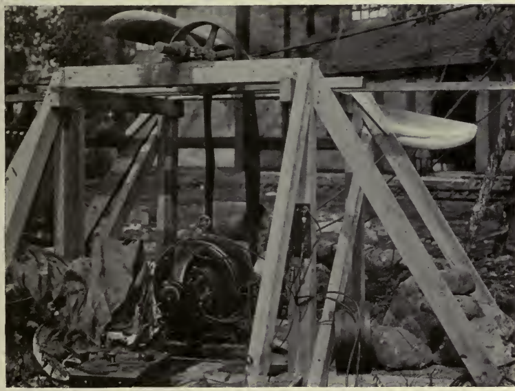
A PERFORATED TANK ABOVE THE SET AND A MOTOR-DRIVEN AIR-PLANE PROPELLER MAKE A SCREEN STORM
