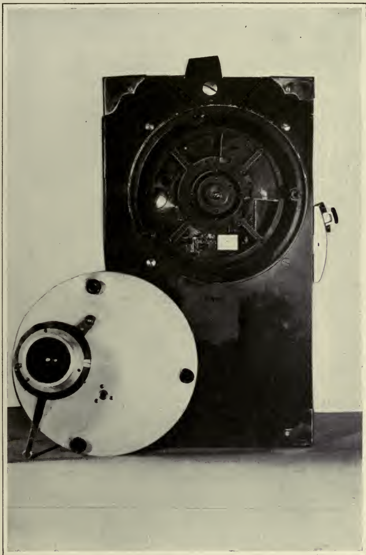
TYPICAL NATURAL-COLOR CAMERA WITH LENS-BOARD REMOVED, SHOWING COLOR-WHEEL AND RAY FILTERS
