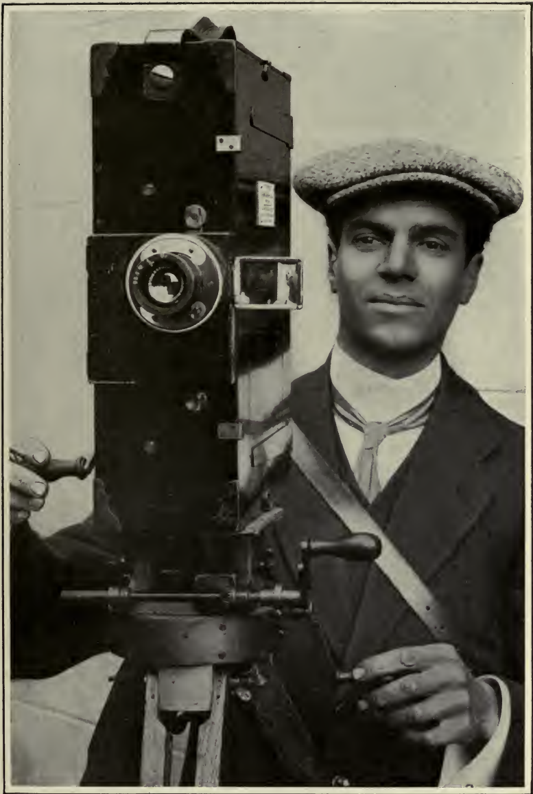
THE PRESWITCH CAMERA, OF BRITISH MAKE, WHICH IS WIDELY EMPLOYED FOR STUDIO AND OUTDOOR WORK
