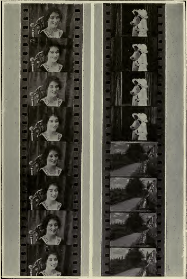
THESE BLACK-AND-WHITE FILMS ARE USED WITH COLOR-WHEEL ATTACHMENTS. NOTE THE DIFFERENCES IN TONE
