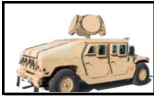
Figure 18. eMHR Mounted on HMMWV. Source: RADA (2016).
