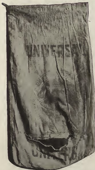
Fig. 3—A poorly mended cement sack showing the use of other material in making the patch. This sack was probably opened by the use of a shovel or knife.
