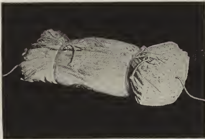
Fig. 7—The first operation in bundling is to bring two of the ropes over the pile, as shown, tying tightly.
