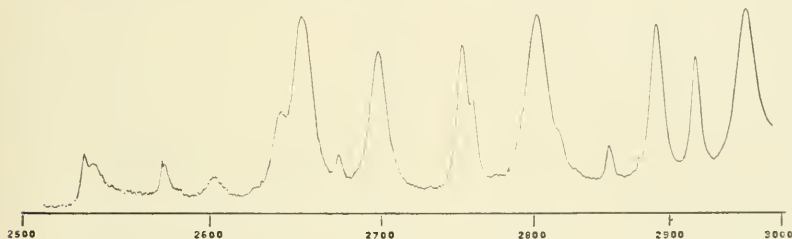
FIG. 5.—Photometric record of photographic spectrogram of mercury arc.
