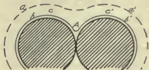
FIG. 37. — Diagram for the explanation of the effect of thickness of water film about soil particles upon ease of capillary movement.
