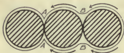
FIG. 36. — Diagram showing the mechanics of the capillary movement of water in soil. The readjustment takes place in the direction of (A) due to the high tension developed by the sharp film curvature at this point.
