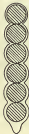
FIG. 33. — Diagram showing the adjustment of the capillary film in a long column and the appearance of free or gravitational water if the weight is too great for the supporting films.
