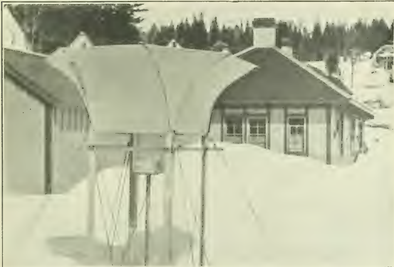
THE MARVIN SHIELDED RAIN AND SNOW GAGE, USED BY THE U. S. WEATHER BUREAU TO MEASURE SNOWFALL. The curved plates forming the sides eliminate the effects of wind currents, thus permitting a true "catch" of snow in the enclosed cylinder.
