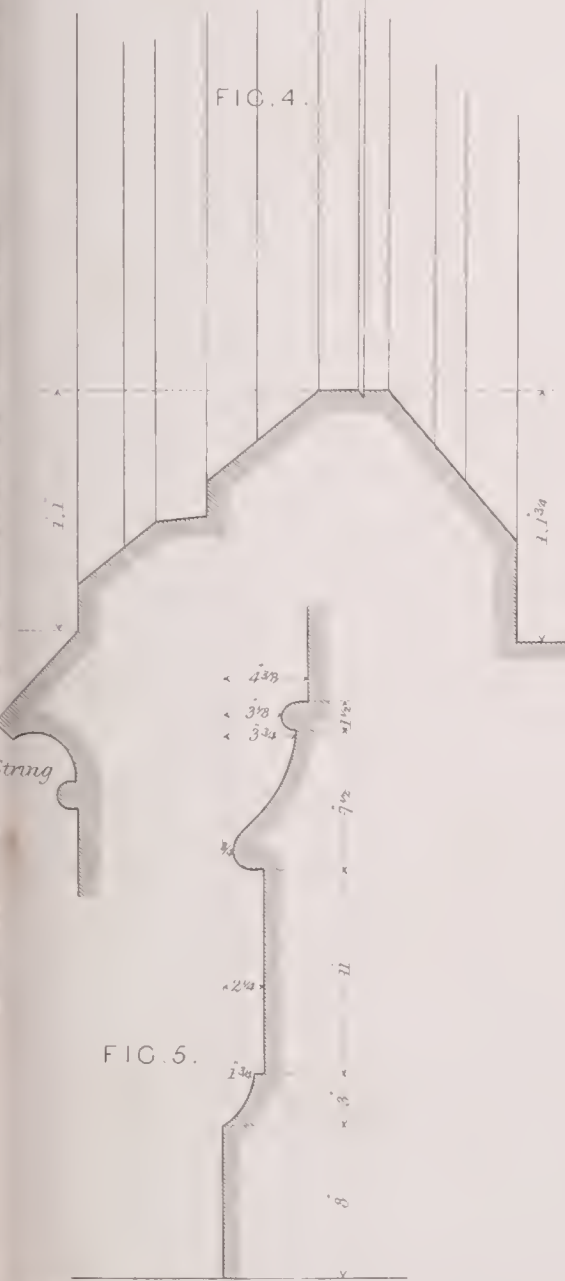
1. Plan of Mullion, Jaumb & label of Window marked B on the Elevation 2. Section thro' Sill 3. Plan & Elevation of Mullion, Jaumb of Window marked A on the Elevation 4. Section thro' Sill 5. Profile of Plinth 6. Profile of Label
