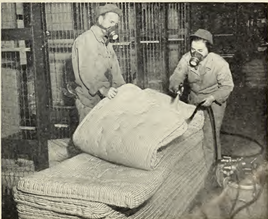
Where a large number of beds must be treated, as in military barracks, a power sprayer speeds up the work. The operators wear masks to prevent the breathing in or swallowing of enough insecticide to be harmful.
