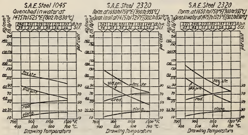
FIG. 19.—Effect of drawing temperature on the tensile properties of steel.
