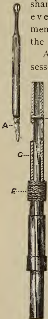
FIG. 2.—The hand piece of the dental engine. A , a bur; B , the support to the instrument; C , slot for fixation; E , the turn-clamp.
