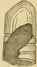
FIG. 1.—Minié ball gnawed by wood-boring larva, nat. size (after C. R. Dodge).
