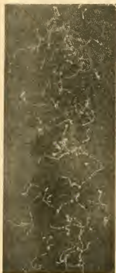
FIG. 7.—Ionisation by X-ray beam about 5 mm. in diameter.
