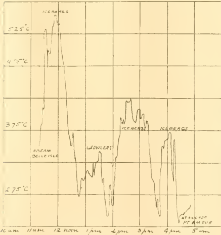
FIG. 2.—Microthermogram through the Straits of Delle Isle, showing the rise of temperature caused by ice.
