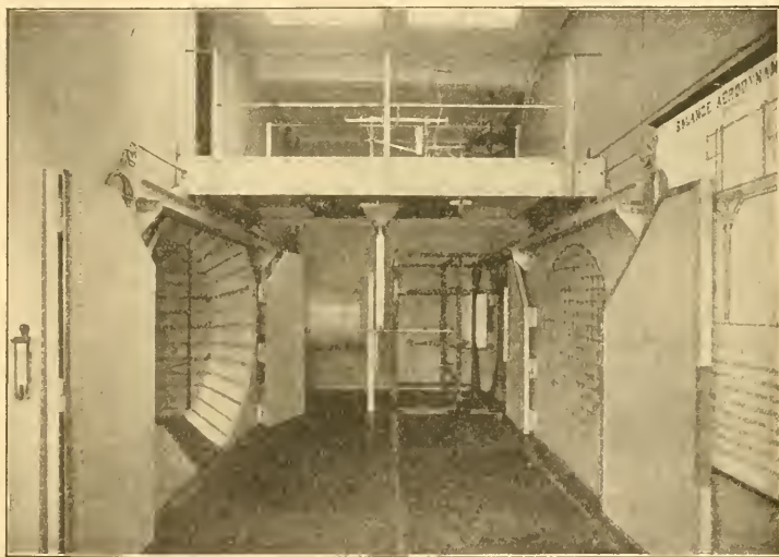
FIG. 1.—Dynamometer room through which the current of air passes from right to left (Auteuil laboratory).
