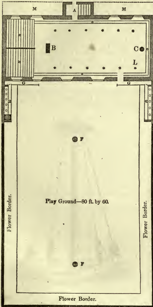
School-room, 60 feet long by 25 wide, and 18 feet high.
