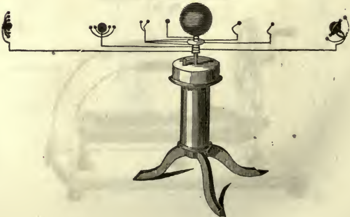
BRASS-MOUNTED SPRING ORRERY. Fig. 20.
