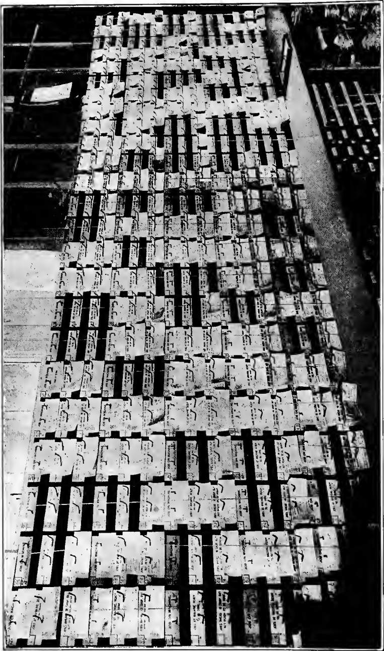
Fig. 2. Bulletin Board of Tabor Mfg. Co. for Controlling Manufacturing Operations and Delivery of Tools
