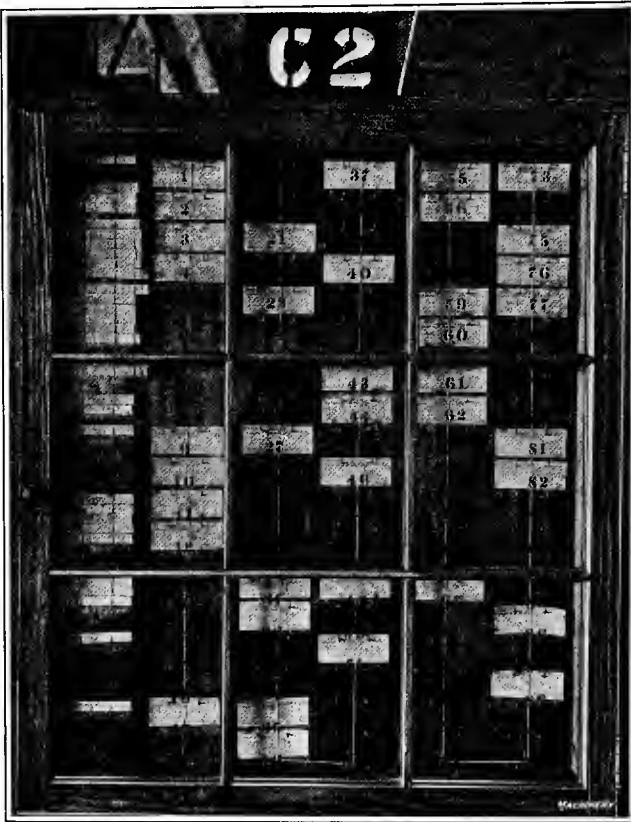
Fig. 3. Shop Bulletin Board which shows Department Foreman what Work is to be done
