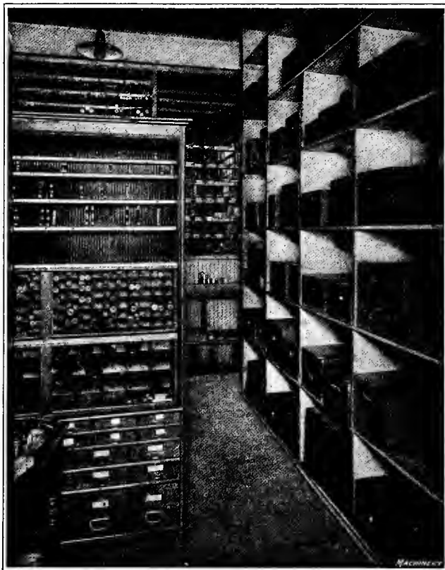
Fig. 2. (Right-hand Section) Storage for Boxes in which Sets of Tools are delivered to Manufacturing Department
