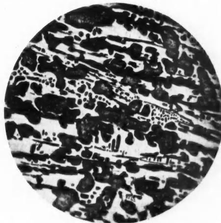
FIG. 5.—WHITE CAST IRON ETCHED WITH CONCENTRATED NITRIC ACID. (Magnified 56 diameters.)
