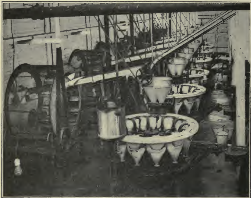
FIG. 6.—A battery of filling machines.
