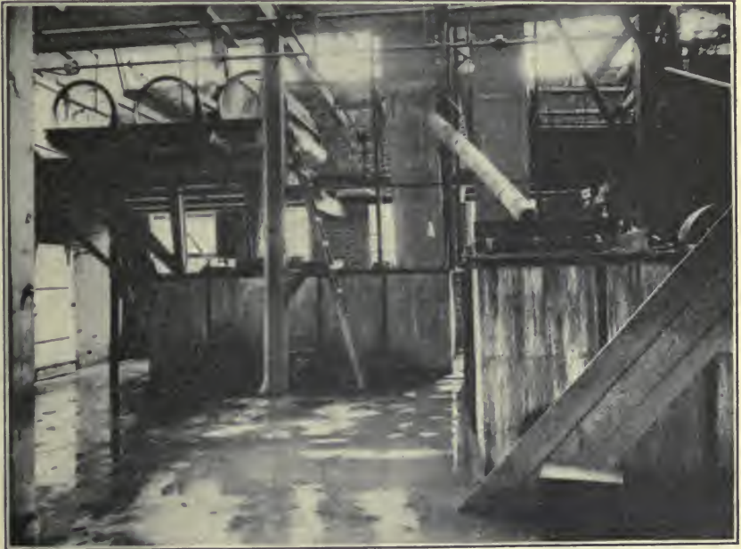
FIG. 2.—Interior of cannery showing squirrel cages for washing peas and the brine tanks where they are graded according to quality.
