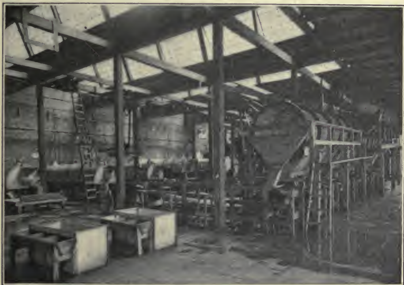
FIG. 5.—A modern sanitary pea-canning plant. The large cylinders on the right are the graders for size. Below them and extending out into the room are the picking belts. On the left are the cylinder blanchers. The roof shows the sawtooth lighting system, and the floor is of concrete for flushing.
