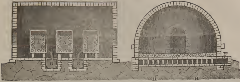
Crystallization and Drying Chambers.
