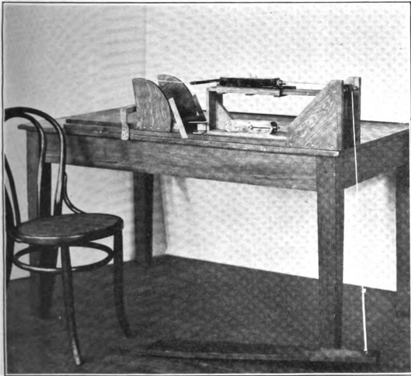
Fig. 1.—Apparatus for testing strength of flexor and extensor muscles in the forearm. The subject to be tested sits in the chair, while the physician uses the pedal attachment in testing the strong flexor muscles of the wrist. The larger registering dynamometer for testing these strong muscles is shown in place on the roller carriage; the smaller dynamometer, for testing the weaker extensor muscles and the finger muscles, is placed below. The nest for the fingers, also not in use, is shown to the left of the smaller dynamometer. The adjustable wooden bar for keeping the wrist down at the same level during flexion and extension is at the extreme left of the apparatus
