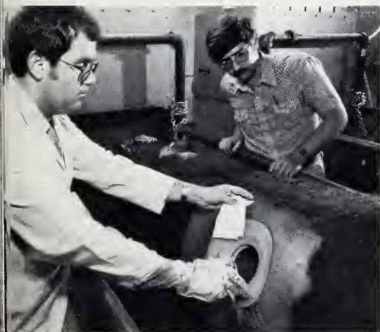
Top: Engineer Ron Montgomery shovels from a draining bin chopped straw treated with alkaline hydrogen peroxide. It will be used—after pressing, drying, and grinding—in a large-scale feed production pilot project. (0783X879-6)
