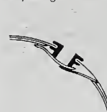
B. Bucket wall deforming to pass gate.
