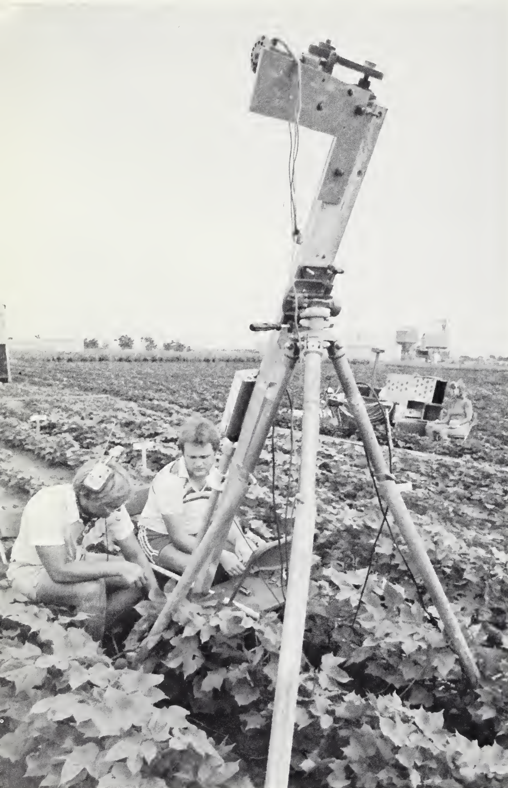
Biological technician Wolfgang Oesterreich (left) and Texas Tech University student assistant Jeff Russell lower a scope into the ground through a plexiglass tube to view the roots of wild Mexican cotton plants. (0882X912-8A)
