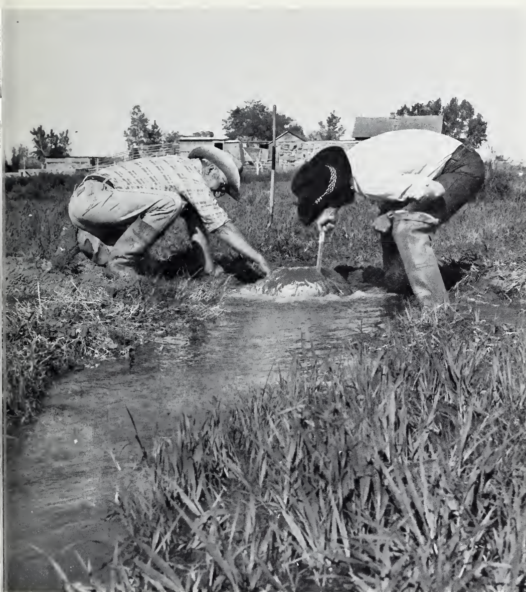
LaBeau (left) and Prestwick measure the flow rate from a riser on the cablegation system installed on LaBeau's farm. The system was designed by ARS and constructed with technical assistance from SCS. (0783X904-1)
