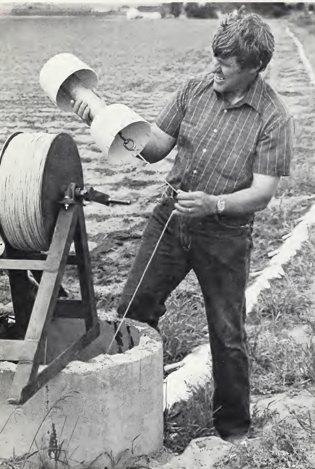
ARS Snake River Conservation Center director W. Doral Kemper, who developed cabling, holds a modified plug that makes it possible to use cabling in an already existing gated pipe irrigation system. (0782X780-36)
