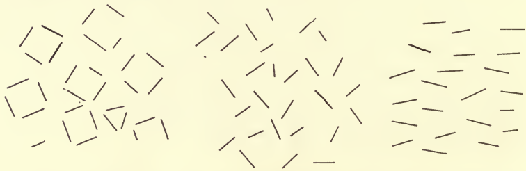
FIG. 27. Diagrams representing molecular magnets arranged in accordance with Ewing's theory of magnetism.
