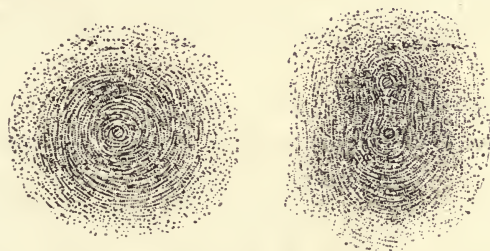
FIG. 26. Diagrams drawn by Faraday showing the magnetic field surrounding one and two conductors carrying current. The particles represent iron filings.
