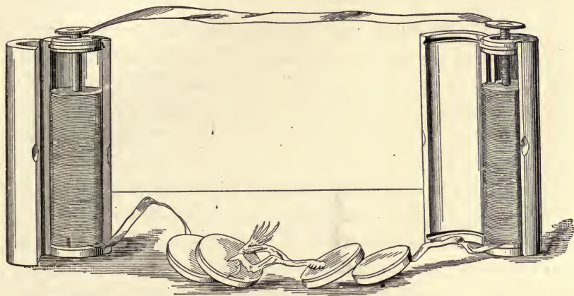
FIG. 15. Volta's electric pile and the "frog-leg" experiment of Galvani repeated by its use.
