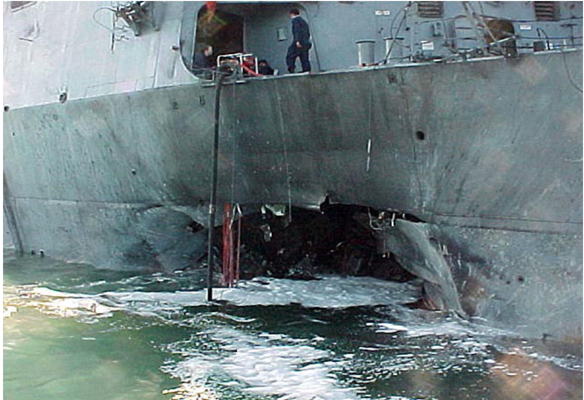
Figure 1. External Damage on USS COLE after Terrorist Attack in Aden Harbor, Yemen October 12, 2000. 17 Individuals were killed in action, 39 were wounded in action. [JMOCN 2002]
