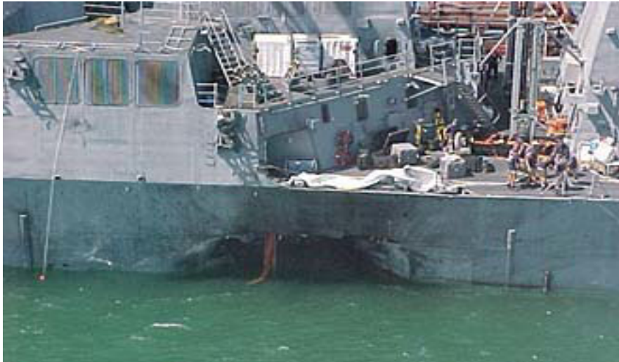
Figure 23. Picture depicting damage to the COLE after the terrorist attack [JMOCN 2002]
