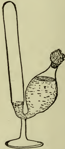
Fig. 247. Fermentation tube filled CO 2 from action of yeast in a sugar solution.
