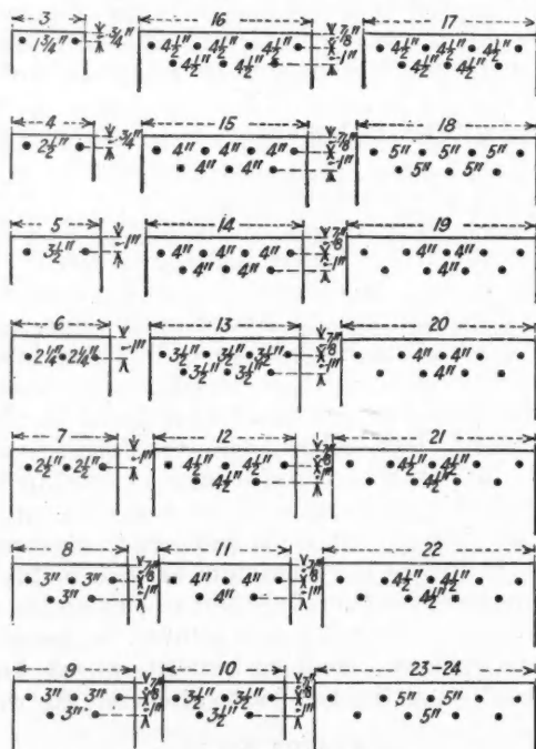
All holes in buckets \frac{5}{8} " for \frac{1}{4} " eclipse elevator bolts. Use one \frac{1}{4} " leather washer on each bolt between bolt and bucket. Width of belt = Length of bucket + 2"
