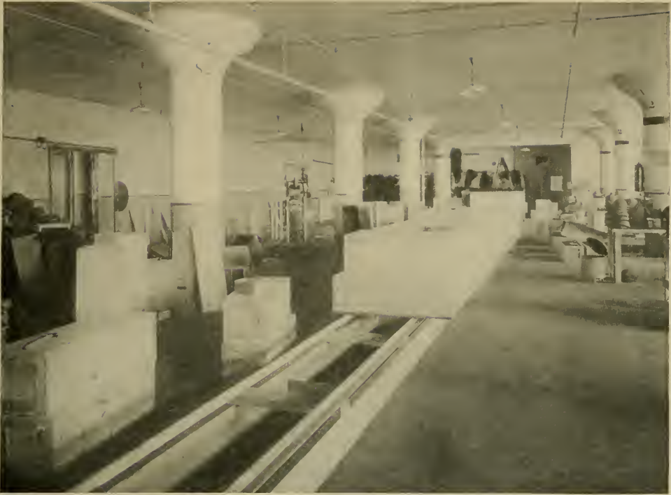
Fig. 160. Cases of British-American helmets passed along a track for storage and shipment
