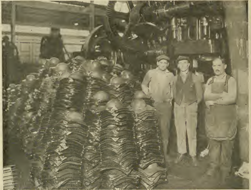
Fig. 144. British-American helmet in process of manufacture. The double-action press, shown in background at the right, stamps out the helmet in a single "draw." Budd Manufacturing Co., Philadelphia
