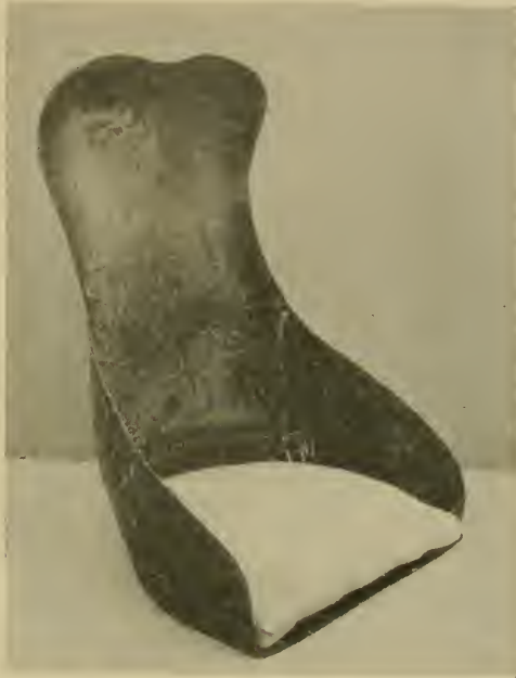
Fig. 213. Aviator's armored chair. Experimental model, American, 1918
