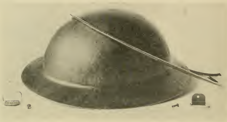
Fig. 146. Manufacture of British-American helmet. Helmet shell, metal rim, chin-strap loops and rivets ready to be put together
