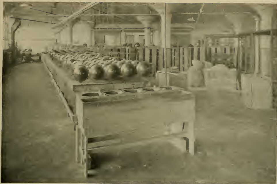
Fig. 154. British-American helmet. Assembling. Freshly painted helmets about to be given a coating of sawdust in the sprinkling box shown in the foreground
