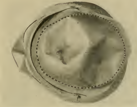
Fig. 169. Experimental helmet model No. 8. Result of test by pistol bullet at 800 f. s. Outline of head within helmet is shown by dotted line. This helmet bears marks of six testing bullets
