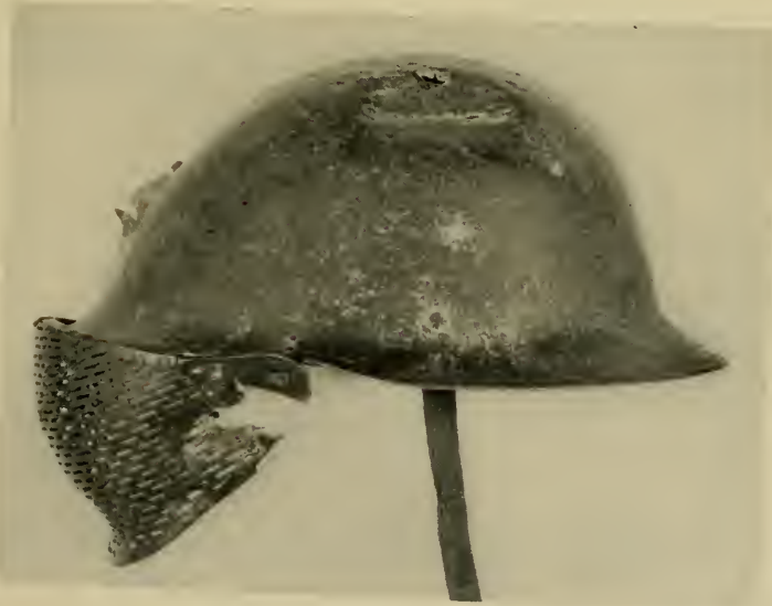
Fig. 48. Dunand helmet, showing result of tests
