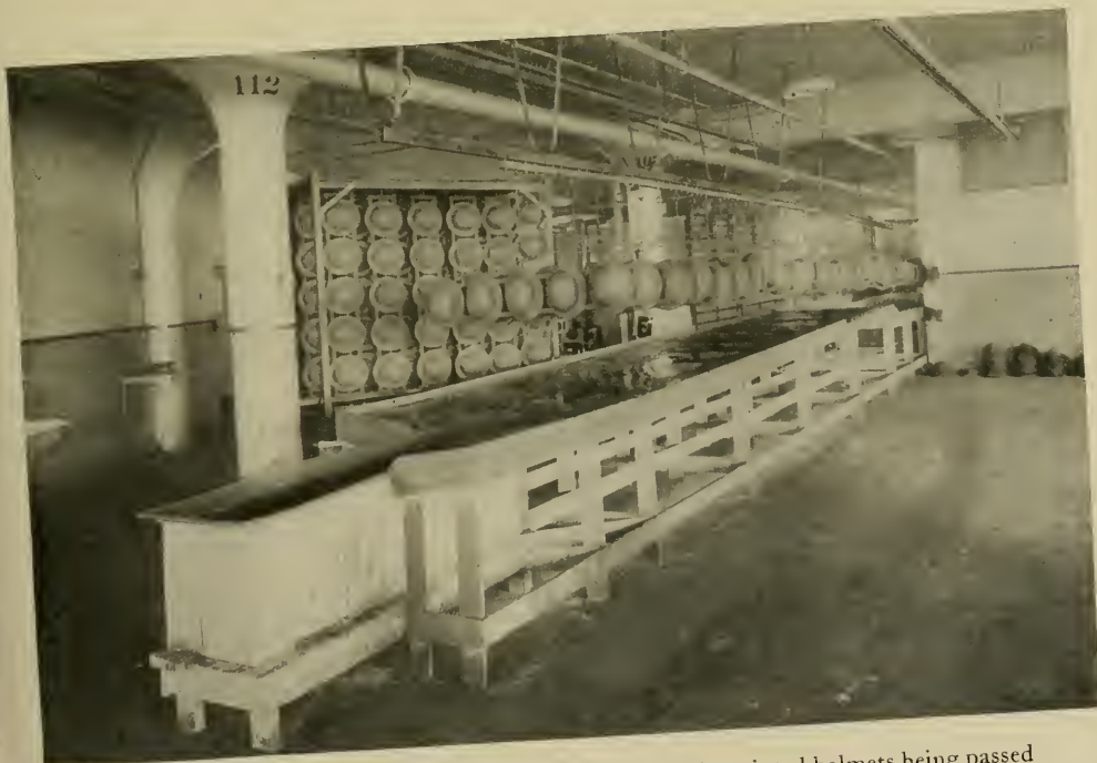
Fig. 152. British-American helmet. Assembling. The helmets are shown arranged in rows on metal racks, front and back, ready to be immersed in the paint trough shown in right of picture. (Ford Mfg. Co., Philadelphia)
