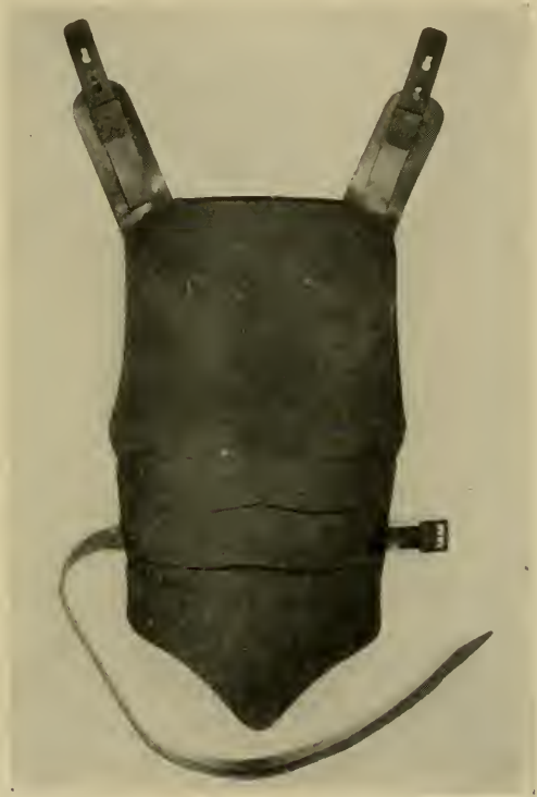
Fig. 198A. Laminated backplate of experimental model, 1918
