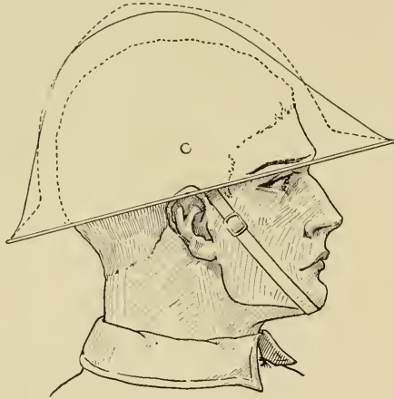
Fig. 181. Liberty Bell helmet. Fall, 1918. Shown over profile (in dotted line) of American experimental helmet model No. 4
