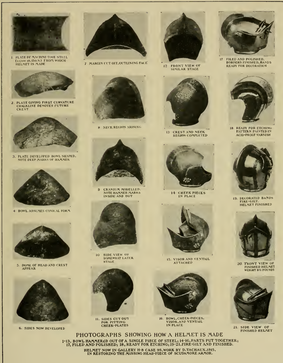
Fig. 7. Stages in making a helmet after the ancient fashion
