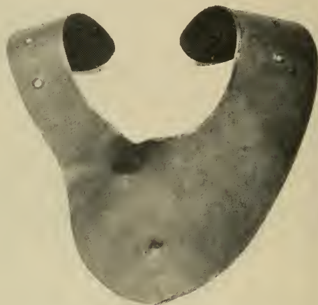
Fig. 190. Similar necklet, showing result of pistol bullet at 850 f. s.
