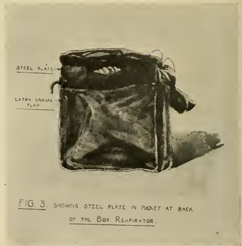
Fig. 203. Drawing provided by British Trench Warfare Division (Captain Rose), showing armored back of box respirator of gas mask. Fall, 1918
