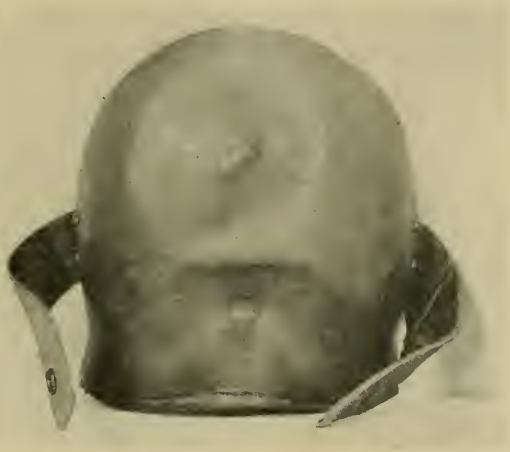
Fig. 188A. Result of test on foregoing face-guard, with pistol bullet at 850 f. s.
