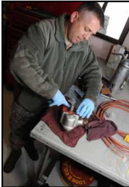
Left: Master Sgt. Chris Asbridge applies lubricant to a part while replacing a cracked thermostat housing on a fire truck.
