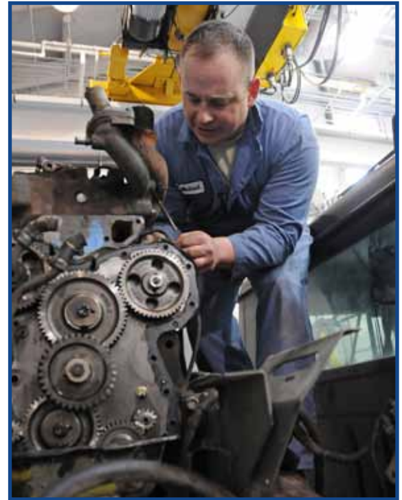
Tech. Sgt. Michael Krouse loosens the bolts on an engine in preparation for removing it.
