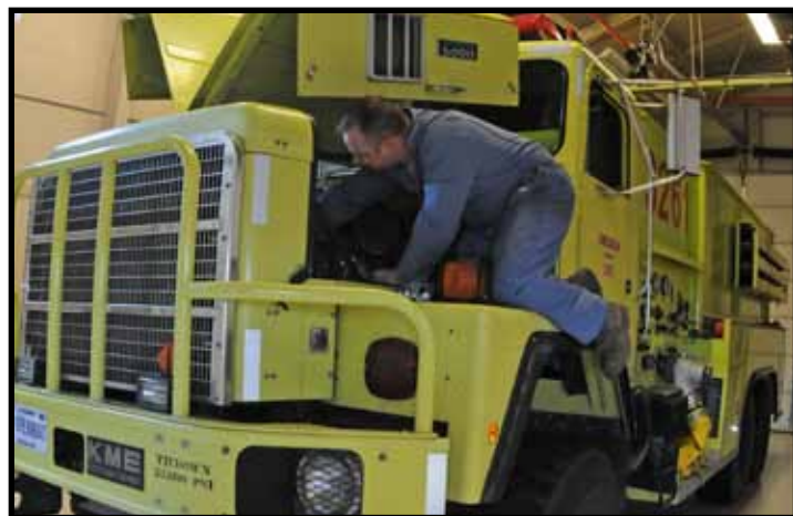
Below: Tech. Sgt. Michael Krouse replaces a cracked thermostat housing on a fire truck
