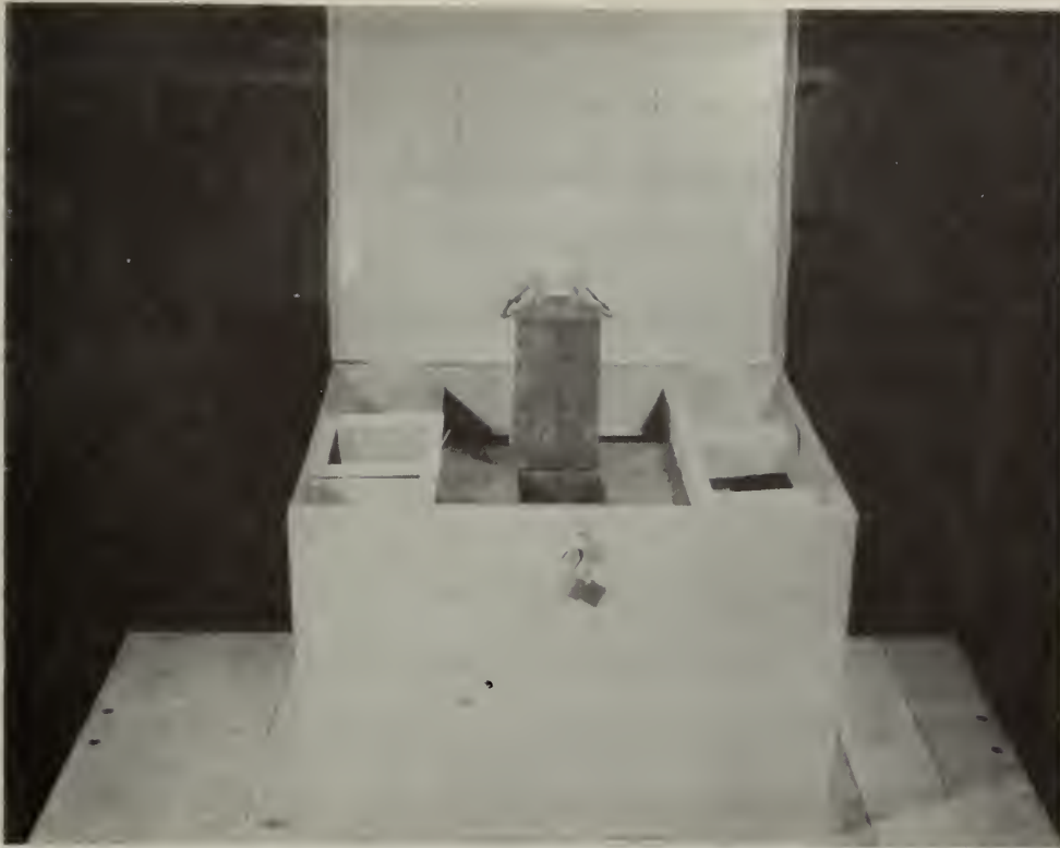
Figure 10 - Source transportation dolly. Shielded volume, 2" deep by 4" square. Shield, 8" thickness lead all directions. Total weight, 2000 lbs.
