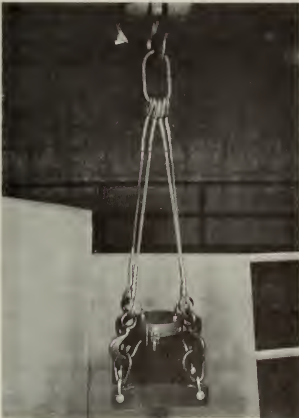
Figure 10 - Source transportation dolly. Shielded volume, 2" deep by 4" square. Shield, 8" thickness lead all directions. Total weight, 2000 lbs.
