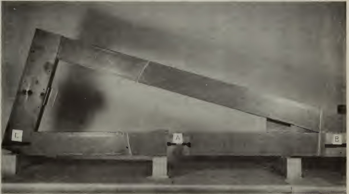
Figure 19 - Spectrograph frame, standing on edge to minimize distortion due to camera angle. Machined surfaces A, B, C are labeled. Reference lines for repositioning the cross over point shield platform are seen between A and C and A and B.
