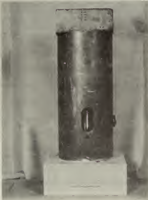
Figure 13 - Assembled source exposure container less the outer steel box. Source removal string at right side.
