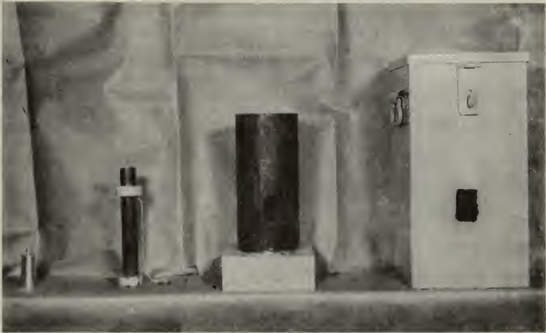
Figure 12 - Source exposure container. Left to right: source, positioning tube, cylindrical lead shield, outer steel box.
