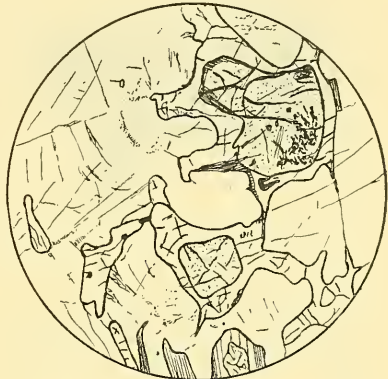
FIG. 2. Section of olivine-gabbro, exhibiting the tendency of the pyroxene to include olivine grains. Section 1103. \times 20 .
