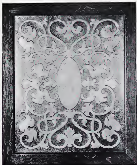
C.—Table-Top, in which the uneven surface of the copper ground is obliterated in the zinc inlay.
