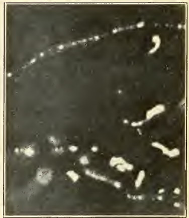
2. RECOIL ELECTRONS. THE X RAYS ARE GOING FROM LEFT TO RIGHT AND THE SHORTER TRACKS PROCEED ALMOST IN THE DIRECTION OF THE X RAYS
