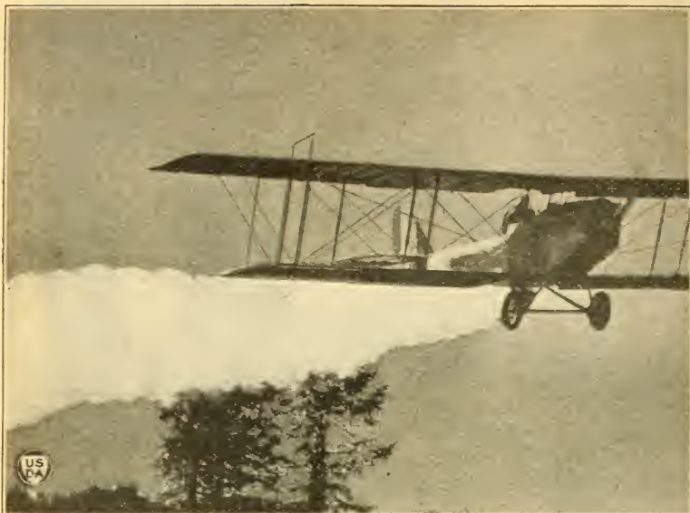
FIG. 11.—Dusting plane in operation, showing behavior of dust as discharged under the body.
