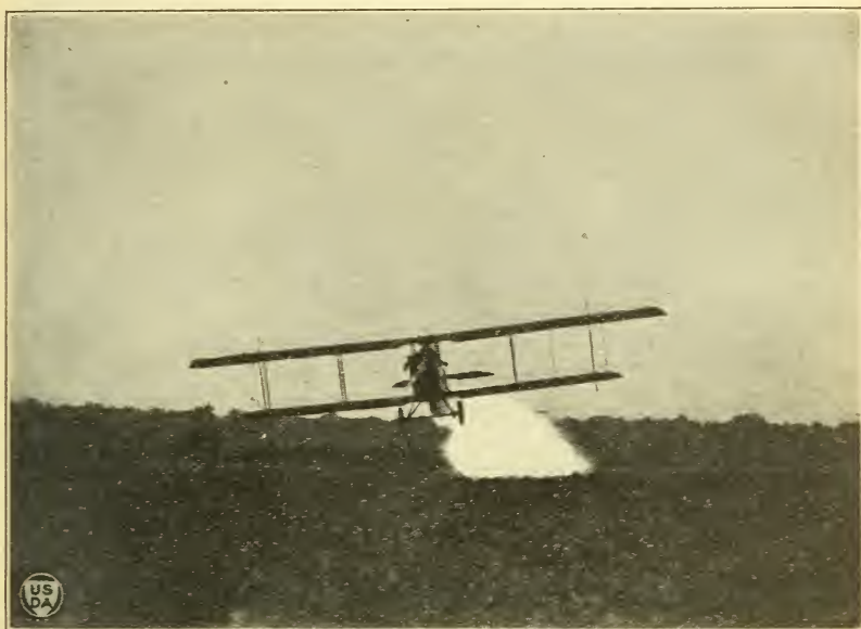
FIG. 13.—Dusting plane directly approaching camera, showing trend of dust cloud. Note how this is blown both downward and to the left of the line of flight of the plane.
