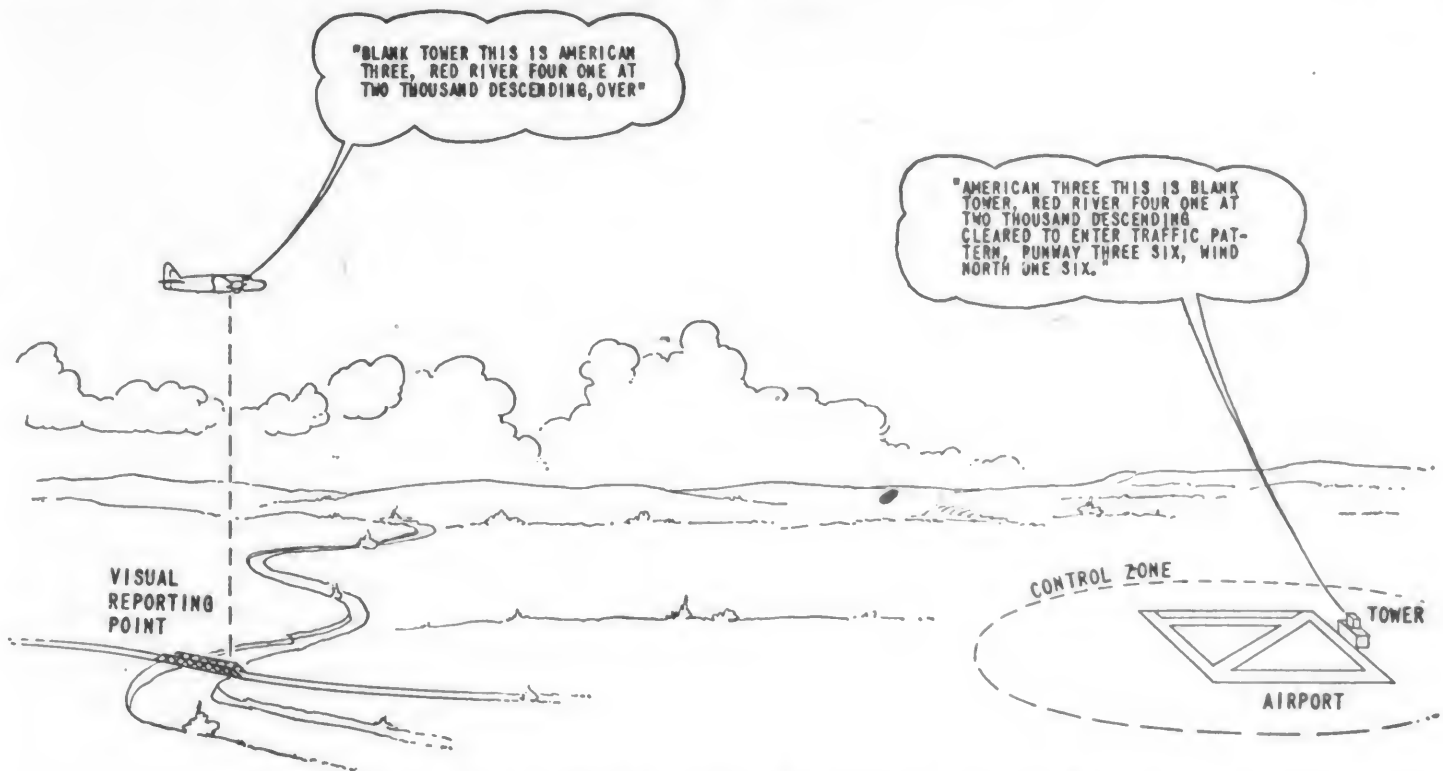
FIGURE 10—Report over a contact reporting point, and clearance to enter traffic pattern.
