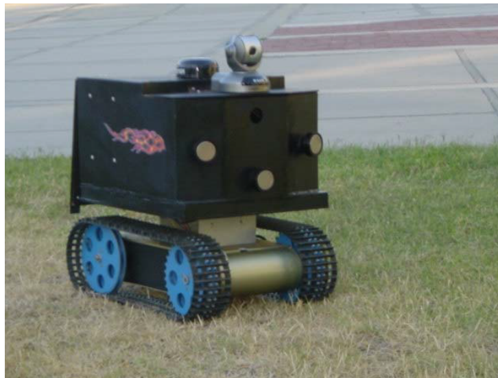
Figure 1.1: NPS robotic platform Bender comprised of a Foster Lemming tracked base and watertight housing for onboard sensors and processing. From [1]
