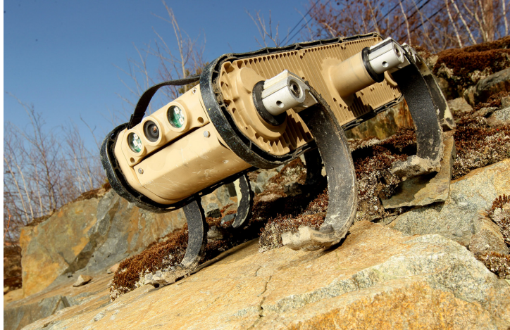
Figure 1.2: The RHex platform from Boston Dynamics incorporating independent drive legs, integrated sensors and durable waterproof body capable of scaling very challenging terrain. From [6]
