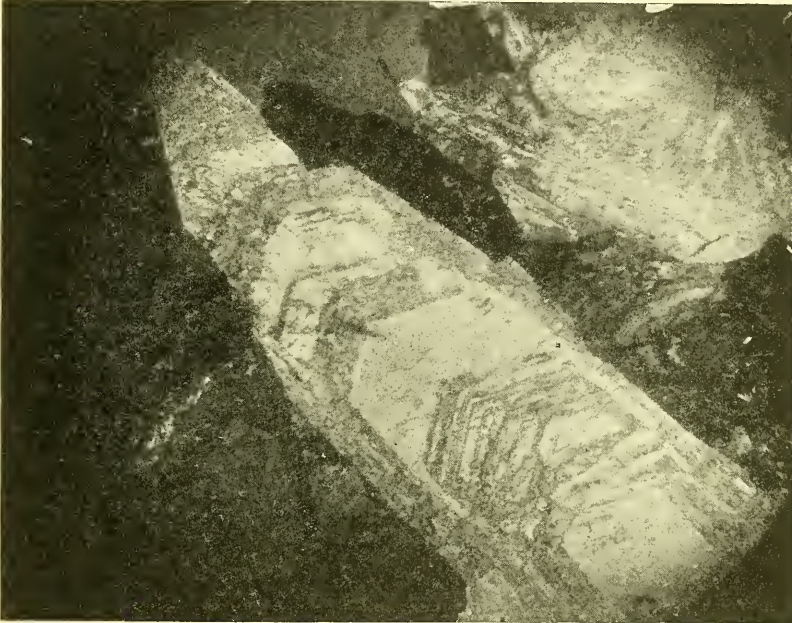
FIG. 3.—Photomicrograph of a section from a pegmatite dike at Flat Rock Portage showing unusual development of zonal structure in sodium-calcium feldspar (crossed nicols; \times 40 ).
