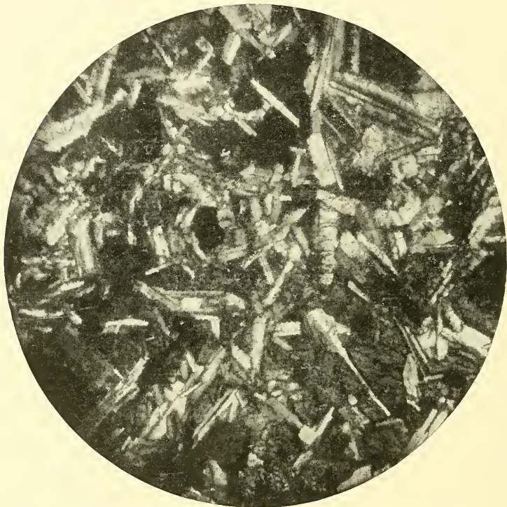
FIG. 2.—Photomicrograph of diabase showing ophitic texture (crossed nicols; \times 40 ).
