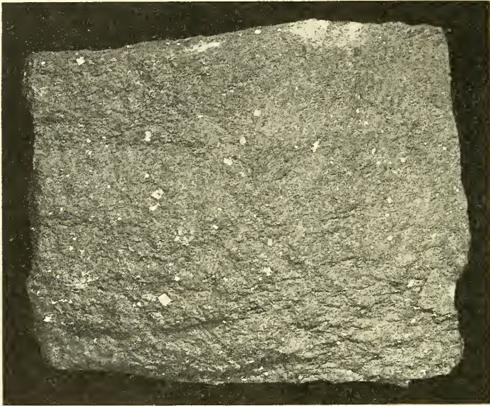
FIG. 1.—Quartz-basalt. \times\frac{1}{2} . The white grains are quartz.
