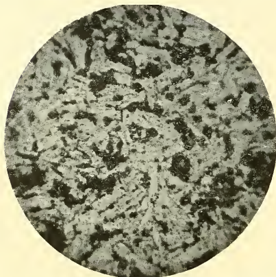
FIG. 9.—Microphotograph of the alkali-feldspar-bearing basalt from Madara-shima. \times 30 .
