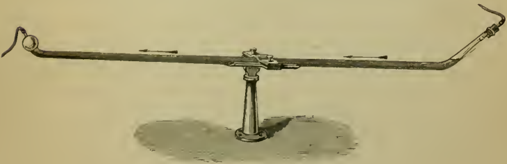
FIG. 252.—Pettenkofer's Tube, for the absorption of carbonic acid gas (§ 98).
