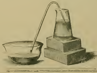
FIG. 333.—Use of the syphon in washing precipitates by decantation.
