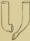
FIG. 218.—Cannulae for aorta and vena cava of frog. The right-hand figure represents the arterial cannula. They are of size suitable for large specimens of R. esculenta (§ 45).
