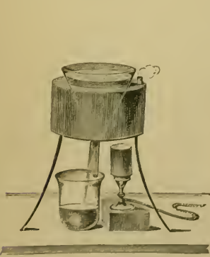
FIG. 336.—Plantamour's funnel for keeping fluids hot during filtration. It may also be used to keep liquids at the freezing point during filtration, by substituting ice for hot water. There are two kinds of these funnels. One of them has simply a wide opening above, and a narrow one below, which is closed by a cork through which the tube of a glass funnel passes. The glass funnel which contains the filter is thus in direct contact with the warm water or ice with which the metal funnel is filled. The other form has a copper funnel in the situation of the dotted line and in this the glass funnel is placed. The glass funnel is therefore only indirectly surrounded by the water or ice on the apparatus, and its temperature can therefore not be so exactly regulated, but it can be removed with great facility and another put in its place, which is not the case when the other form is employed.
