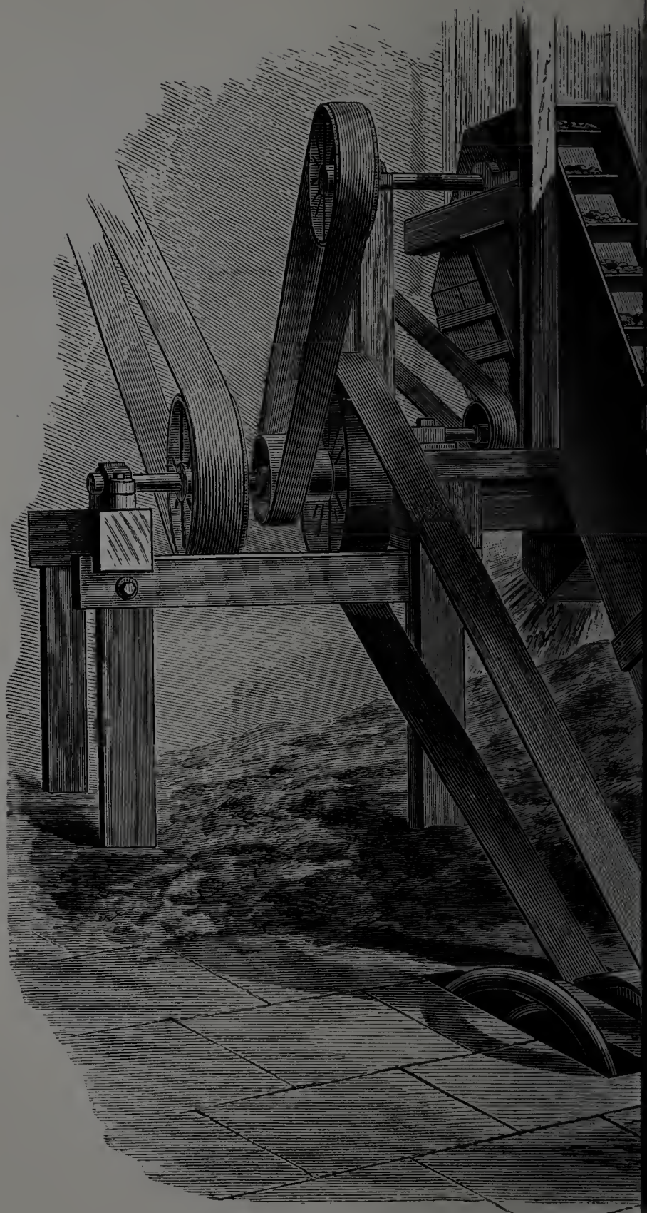
FIG. 50. MILL FOR PREPARING THE CLAY, A
