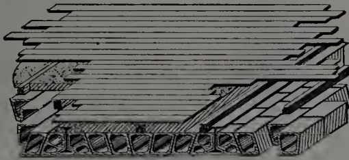
View of 9 in. Tile Arch, between 10 1/2 in. I beams. Weight 38 lbs. per square ft.
