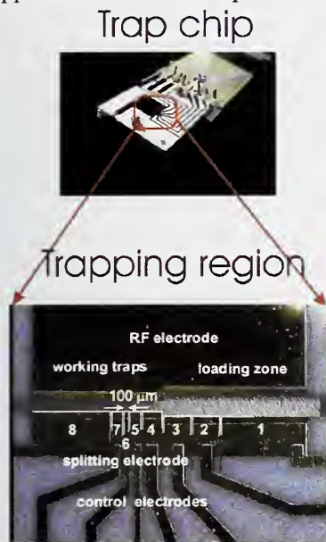
Figure 2. Six-zone alumina wafer ion trap The team is conducting research on developing traps to support two-dimensional ion arrays to support more efficient quantum computing with larger numbers of qubits.
