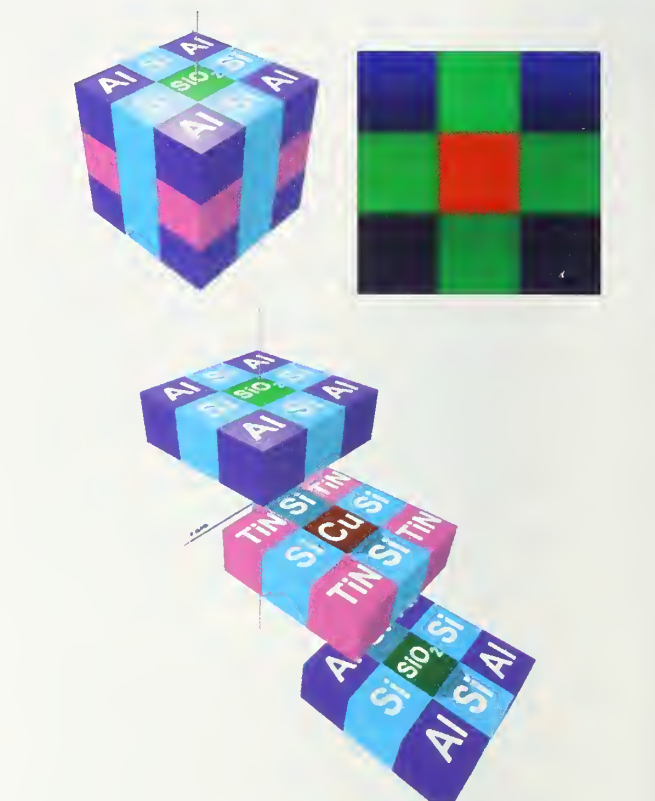
Figure 2. (top left) Phantom sample consisting of a "Rubik's cube" of aluminum, silicon, silicon dioxide, titanium nitride, and copper. This fictional sample contains many of the materials used in modern semiconductor devices, admixed and juxtaposed on the nanoscale to simulate the complexity of true 3D chemical imaging problems. Each of the 27 smaller cubes is 100 nm on an edge, so the entire assembly is 300 nm on an edge. The beam (purple vertical line) is shown striking the sample in the center of the \text{SiO}_2 subcube. (top right) 3-color X-ray elemental map showing quantitatively the detected X-ray intensities for the Cu K\alpha X-ray emission line (red), the Si K\alpha X-ray emission line (green), and the N K\alpha X-ray emission line (blue) after excitation with a 20 keV incident electron beam. Note the differential absorption of the Nitrogen K line from bottom to top (the X-ray detector is off the top of the image) and the bleeding of excitation near the phase boundaries. The X-ray map is 300 nm on an edge. (bottom) The same cube shown with the top, middle, and bottom layers vertically expanded and horizontally translated to reveal the 3D structure more clearly.
