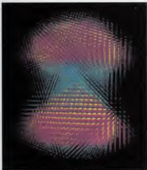
Figure 2. Atomic-scale charge density of a typical electronic state in a double-dot molecule.
