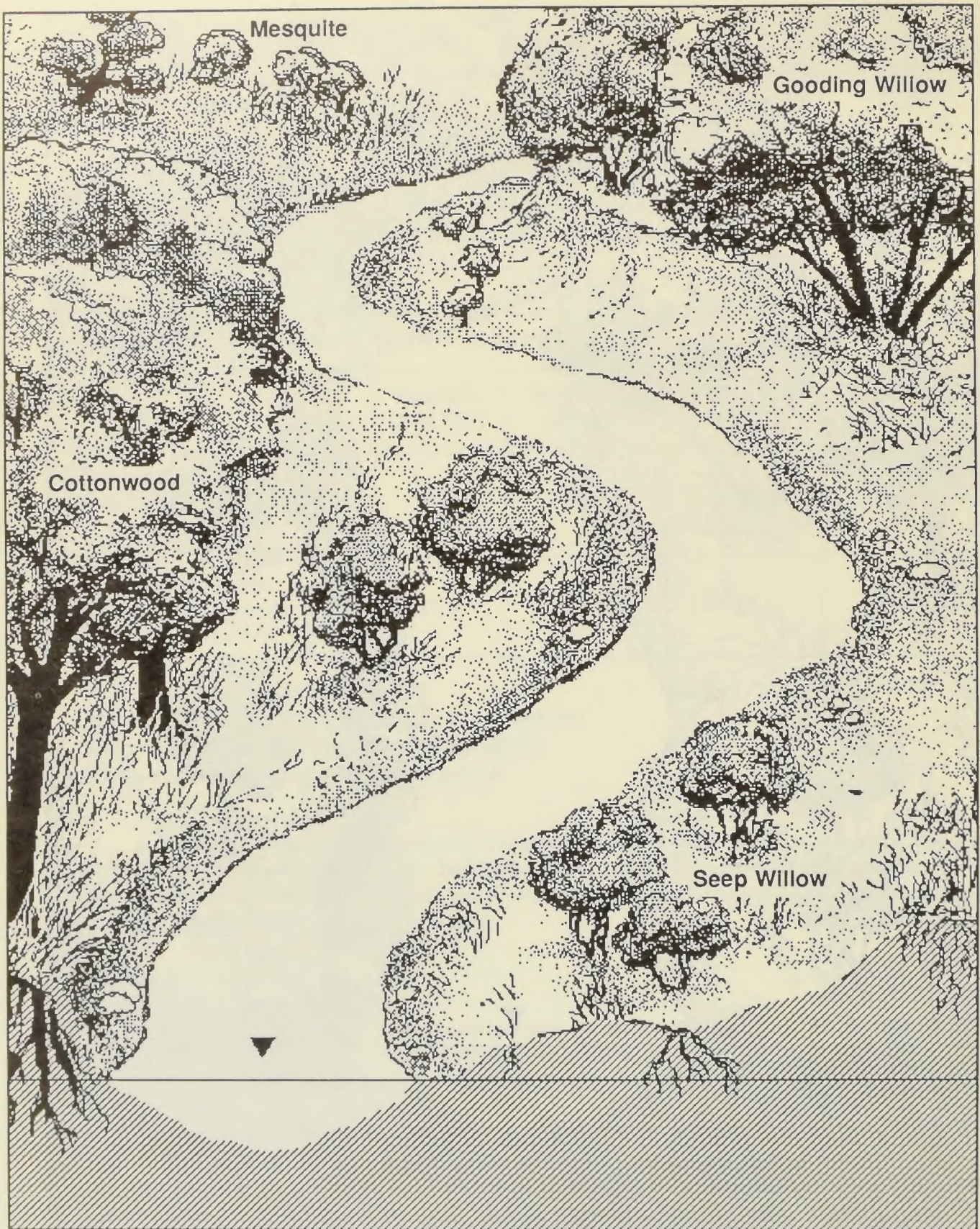
Figure 5. Depiction of riparian vegetation position and relationship to ground water on a typical channel bend.
