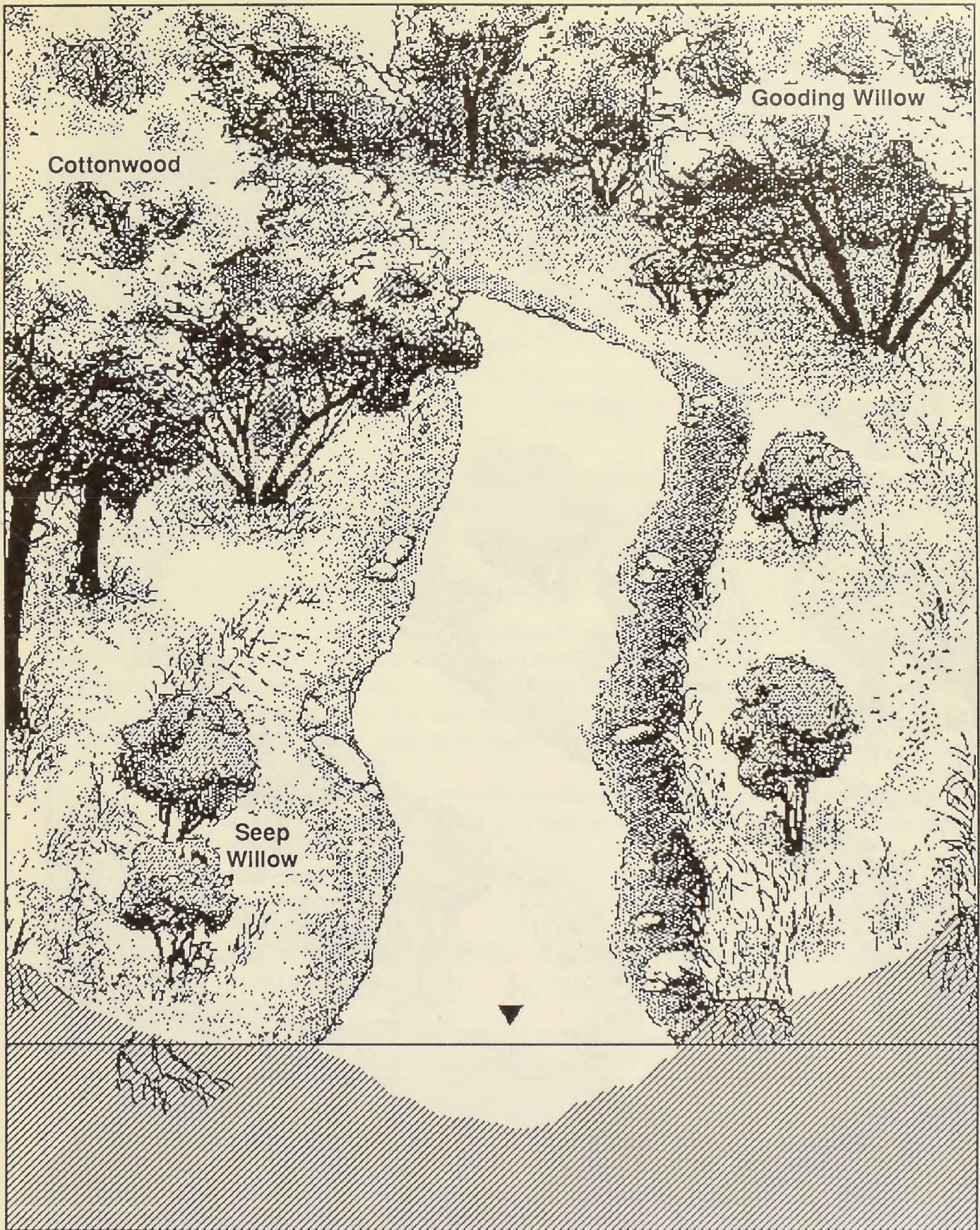
Figure 4. Depiction of riparian vegetation position and relationship to ground water on a typical straight Channel reach.
